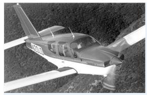
**STANDARD DATA:** Seats 4. Gross wt. 3,086. Empty wt. 1,763; (TC) 1,850. Fuel capacity 86. Engine 250-hp Lycoming 10-540 (TC) 250-hp Lycoming TIO-540.
