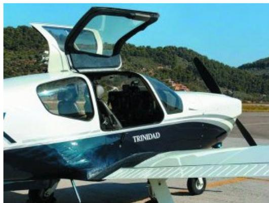
*The door sill is higher than on a Piper or Beech, but the large opening helps ease boarding.*
