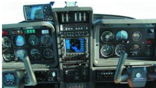
*Modular panel has right-side gauges angled to face the pilot.*
