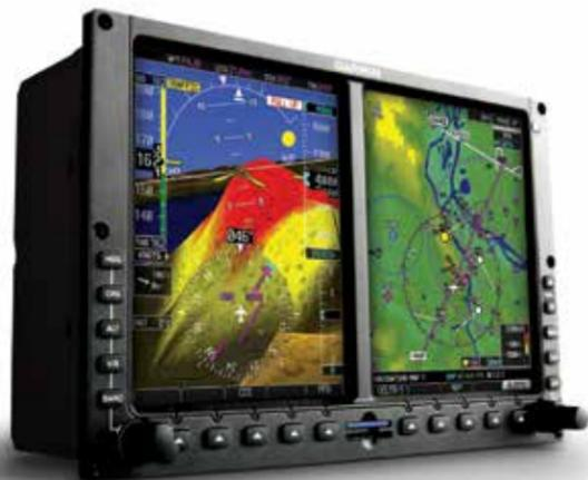
A scaled version of Garmin's SVT™ 3-D synthetic vision renders terrain-alerting data into a realistic virtual landscape, showing obstacles, traffic, airports and more. SVT is standard on G600; optional on G500.
