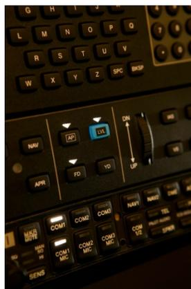
Also unique to Garmin is a blue “LVL” button on the GFC 700 autopilot mode controller. The LVL button is a pilot’s get-out-of-jail-free card when things are starting to go bad. Simply push the LVL button and no matter what mode the
