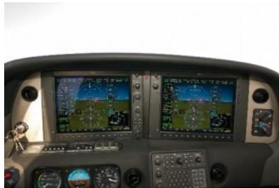
The Perspective panel is not just another G1000. Unique to Cirrus, at least for now, are impressively large dual 12-inch displays. The primary flight display features Garmin’s recently announced [synthetic vision technology \(SVT\)](#) and several crew alerting messages.
