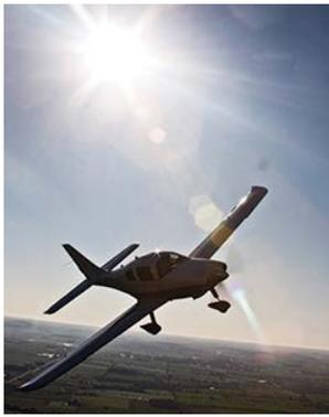
*The all-composite Cessna 350, powered by a 310 hp Continental IO-550N engine, is the first Cessna single to extensively use bonded composite structures.*
