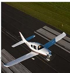
Like the Cirrus SR22, the Cessna 350 relies on a combination of copious power and extreme aerodynamic cleanliness to overcome drag. Officially, the airplane's max cruise speed checks in at 191 knots, but that's probably not the way most pilots run the 350. The penalty for big cruise is big fuel burn, not very popular at a time of \$6-per-gallon gasoline.
