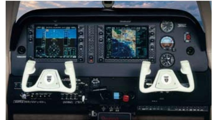
A picture is worth a thousand words. And the Garmin G1000's twin 10.4-inch, high-resolution liquid crystal displays speak volumes about the system's ability to deliver more information in a way that's intuitive and easy to understand. Primary flight information, engine performance, graphical navigation, available traffic, terrain and XM satellite weather — it's all here. Even integrated Garmin autopilot, barometric VNAV and WAAS with LPV approach.
