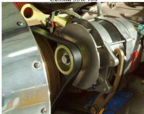
One of two 70 amp alternators Cessna 350/400
